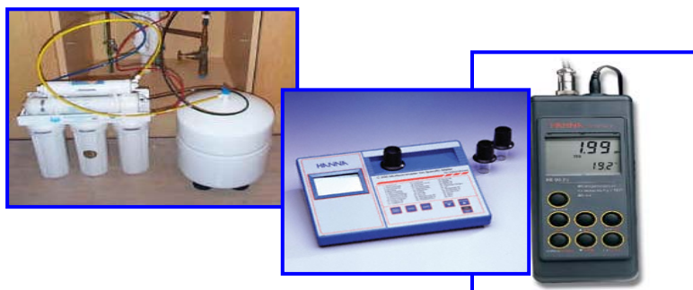
Figure (3-15): Models of the equipment added to the desalination technology lab, Faculty of Engineering, Alex. Univ. (C-096-H0)
